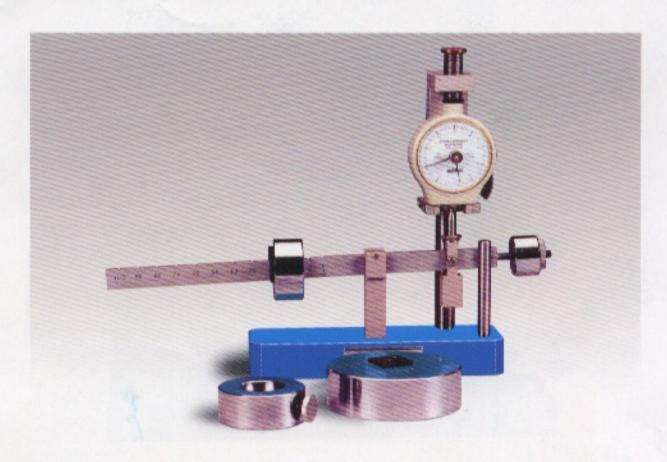
The Instrument is useful for the routine check of the reading accuracy of Shore A & Shore D Rubber Hardness Testers to comply with applicable standards DIN 53505 & ISO R 868, BS 903 Part A 26.
